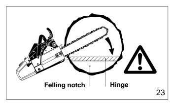
Then, determine the placement of the felling notch (fig. 21). The felling notch when properly placed determines the direction in which the tree will fall. It is made perpendicular to the line of fall and should be as close to the ground as possible. Cut the felling notch to a depth of about one-fifth to one-fourth of the trunk diameter (fig. 22). It should be in no case higher than it is deep. Make the felling notch very carefully.
